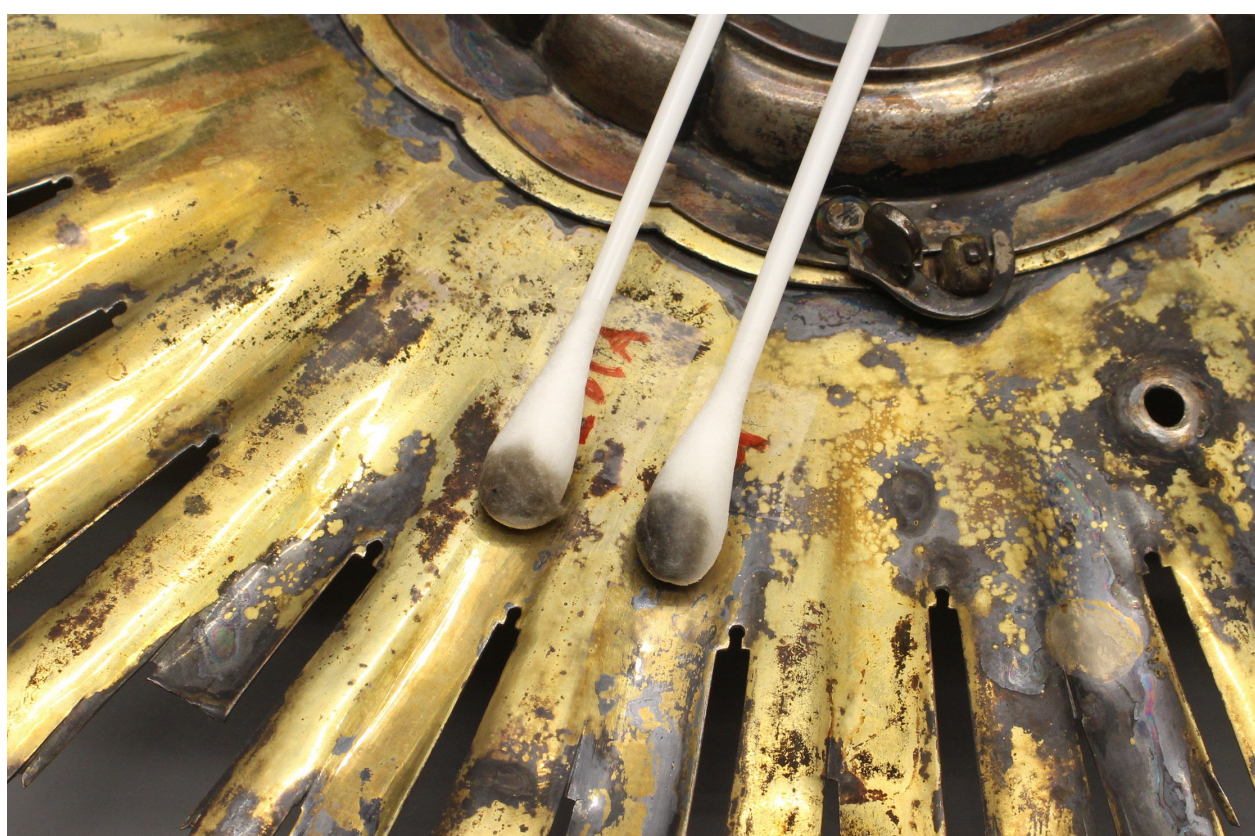
Photo: Removal of copper and silver corrosion products from the gilded rays of an 18th-century Baroque monstrance Collection: Slovene Museum of Christianity, Stična (photo: Nataša Nemeček)
